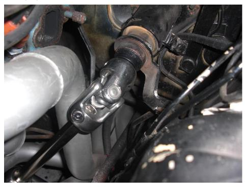
16. Verify that your rack is centered and set your toe adjustment by eye trying to keep the front wheels straight. Once you have this done install your steering wheel in place and tighten to 30 lbs ft. Reinstall the horn pad and take the car to a professional for an alignment. Enjoy the drive.
