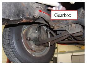
8. Remove the stock round crossmember from the vehicle and install the rack and pinion assembly in its place. Use the supplied bolts to put it in place and tighten to 65 ft.lbs.
