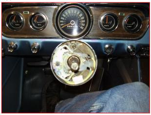
3. From under dash remove the bolts that retain the column tube to the dash. Remove the 3 screws at firewall where the column goes through and remove retainer plate.
