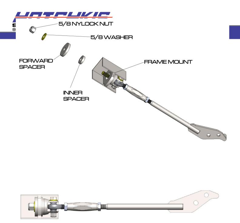
7 *Install Lower Control Arm Mount* Tighten up the supplied nuts & bolts for the lower control arm mounting point and you are done.
