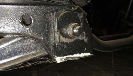
Install Hotchkis Arm Inner Mounting Point Grab your Hotchkis lower control arm and reinstall in the same manner as removal.
