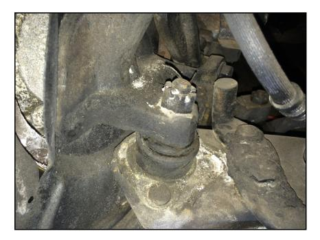
The ball joint stud is taper pressed in the spindle mount. To remove the stud from the spindle force and/or impact is required to break the press fit. There are a number of ways to do this, but the best method is to make an inexpensive tool with
