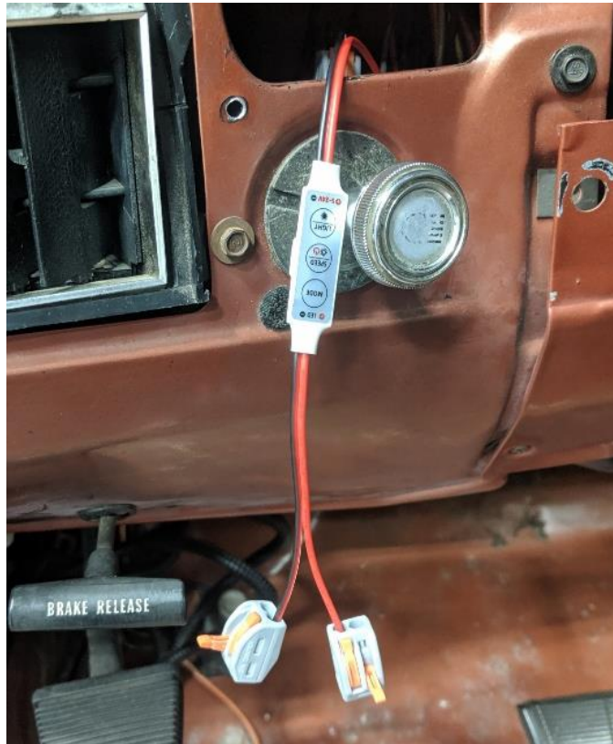
Figure 12 - Install Connectors to LED Dimmer
