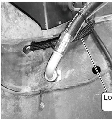
Loom and secure excess wire
