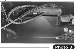
Connect wiring harness to corresponding port on ECU
