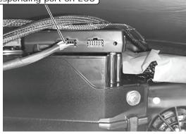
Route wiring harness from A/C control knobs behind dash to glove box area
