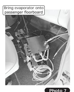
Run heavy gauge orange and white wires through grommet
