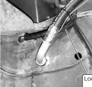
Loom and secure excess wire
