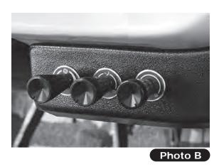
Vintage Air also offers an **optional upgrade control panel kit** for the 1961-64 Ford F-100 that features our stylish Streamline control panel (See Photo C, below). Available in both Polished and Black Anodized, it may be installed at the time of system installation or retrofitted anytime thereafter with a simple modification to the center louver bezel. **NOTE: Additional purchase of Vintage Air Kit** # **491644 or 491645 is required. See bit.ly/vapanelupgrade for installation instructions.**
