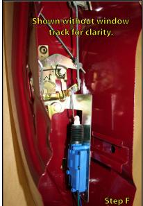
Image shown without latch or window track in place to illustrate placement of bracket.
