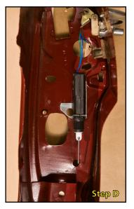
Image shown without latch or window track in place to illustrate placement of bracket. Latch removal is not necessary.
