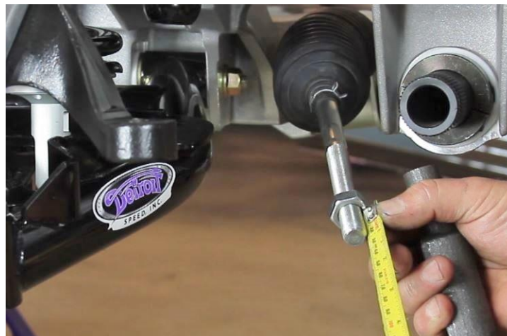
Figure 38 – Install Outer Tie Rods
