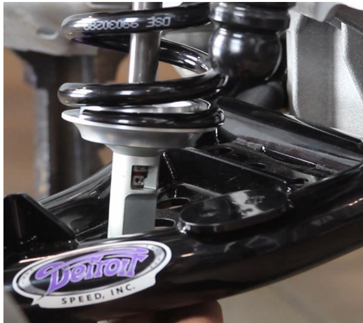
Figure 33 - Lower Coilover Mount
