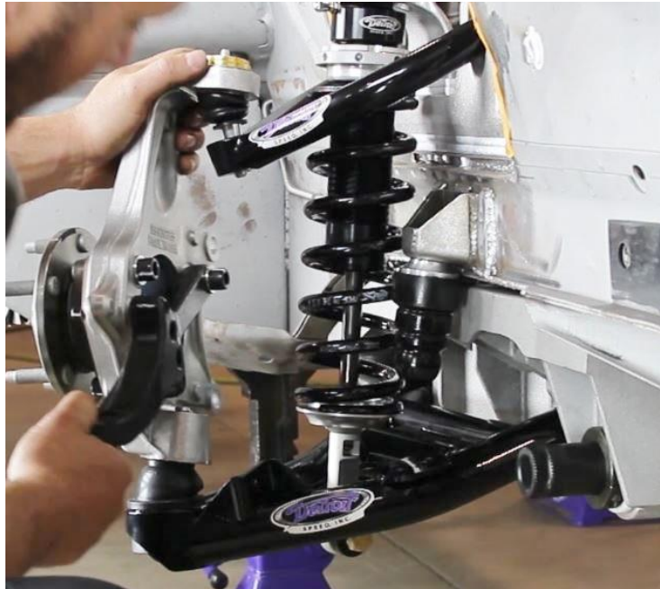
Figure 34 – Install Spindle Assembly
