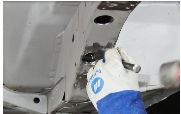
Figure 8 - Drill-Out Bottom Frame Rails
