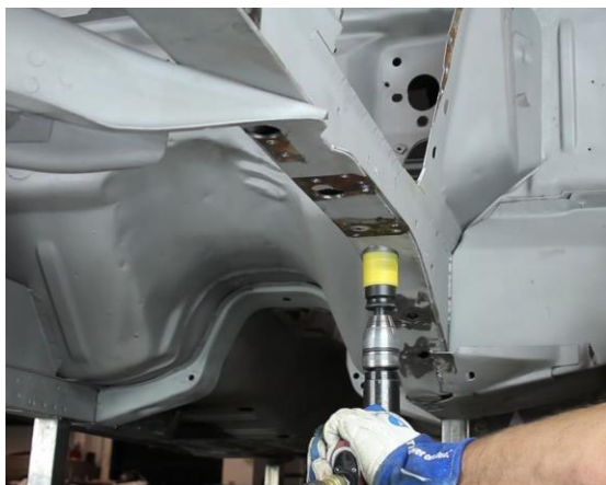
Figure 8 - Drill-Out Bottom Frame Rails
