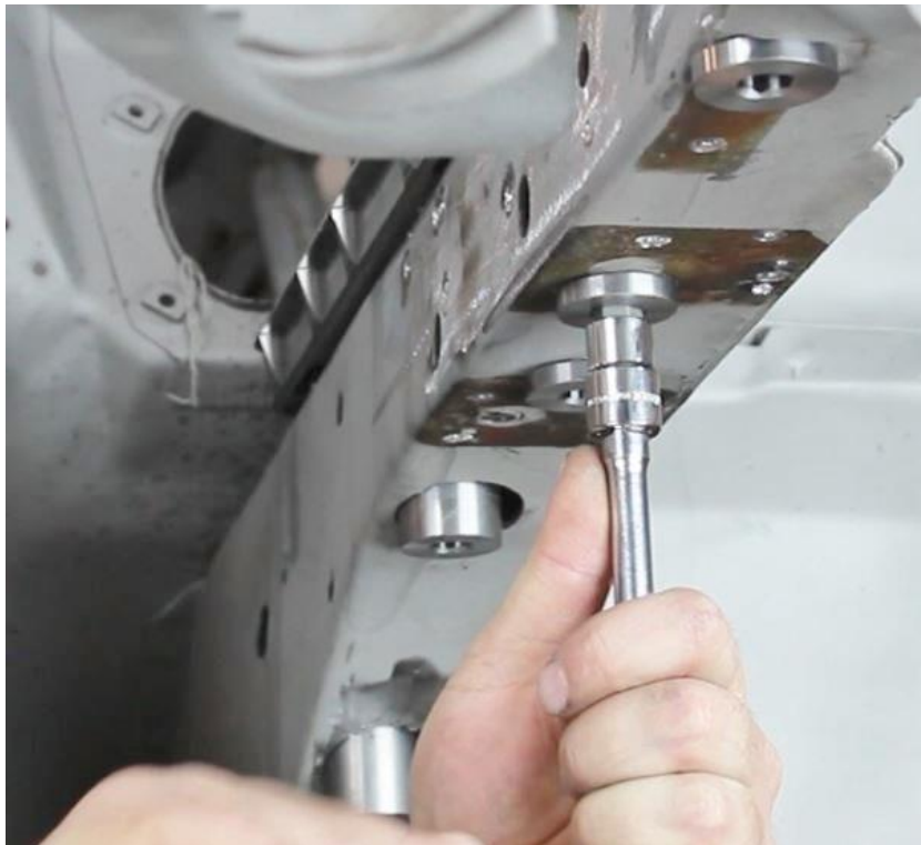
Figure 14 - Tighten All Floating Stanchions Sleeves
