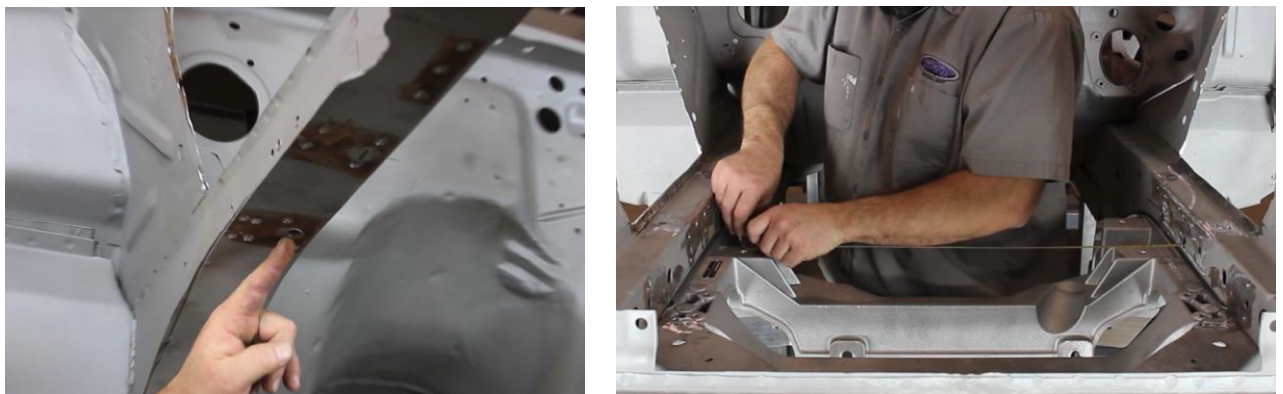
Figure 6 – Locate Aluma-Frame Cradle
