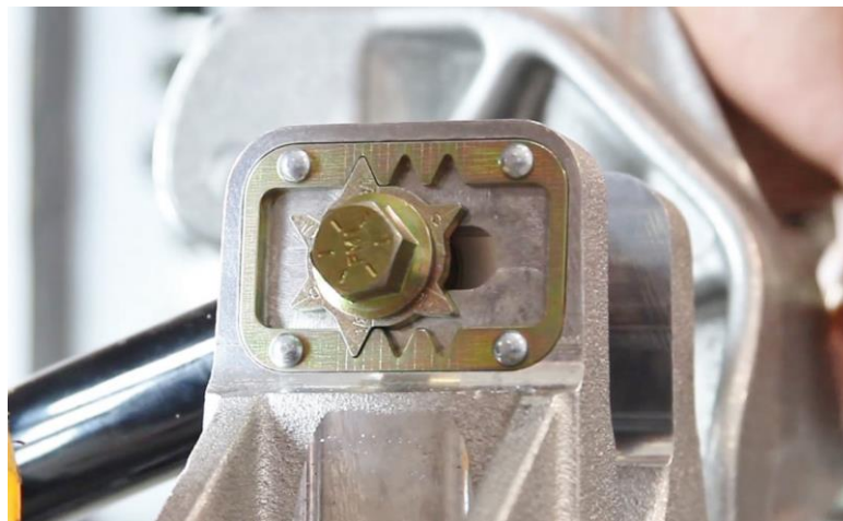
Figure 28 – Install Upper Control Arms
