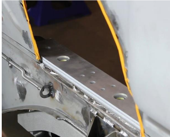
Figure 24– Install UCA Bracket Shims
