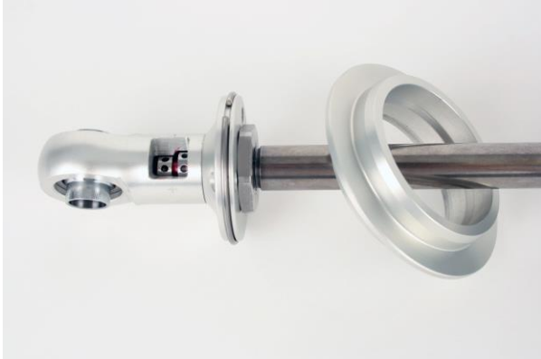
Figure 29 - Remove Upper Spring Seat
