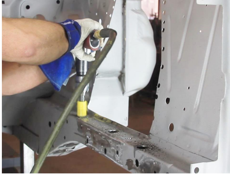
Figure 9 – Drill-Out Top Framerais
