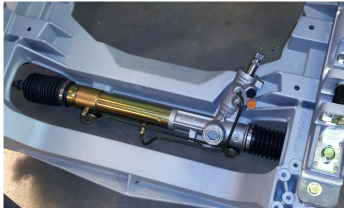
Figure 37 – Installed Rack & Pinion
