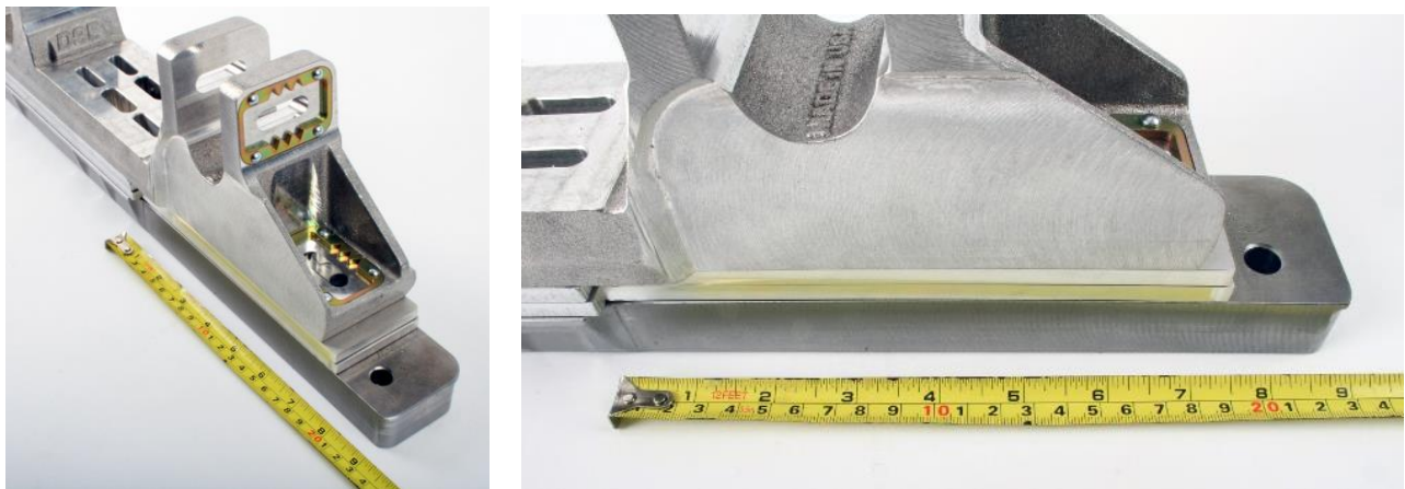
Figure 5 – Modify Frameraill Adapter, Adjuster Shims & UCA Mount
