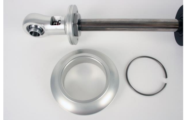
Figure 30 - Upper Spring Seat & Retaining Ring
