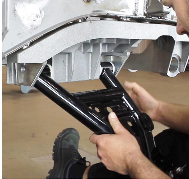
Figure 20 – Install Lower Control Arms
