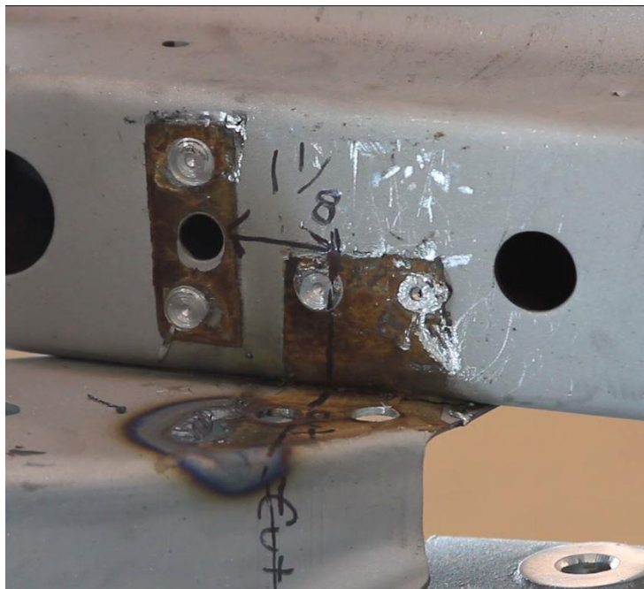
Figure 4 - Trim Framerail Brace
