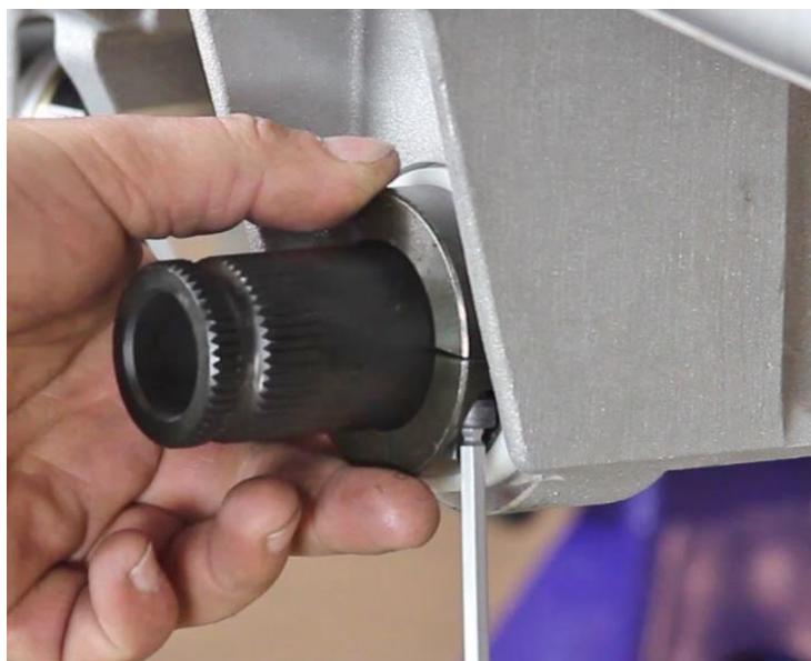
Figure 23 – Install Split Lock Collars
