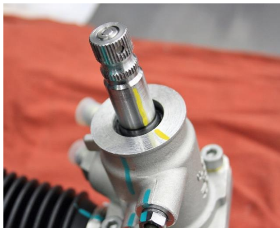
Figure 35 – Center the Rack & Pinion
