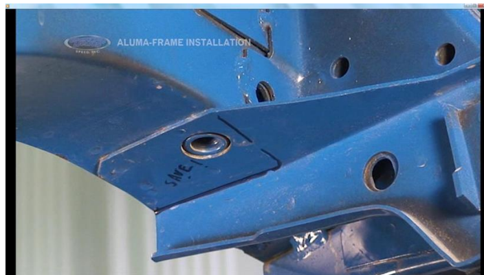
Figure 1 – Remove Factory Brackets
