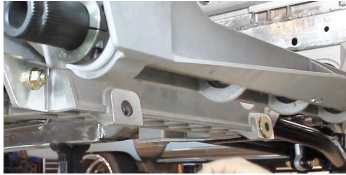
Figure 36 – Install Mounting Spacers
