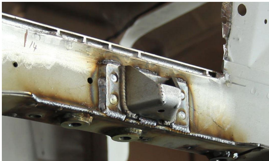
Figure 19 - Weld Jounce Bumper Bracket
