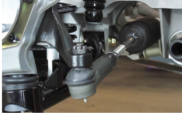
Figure 39 - Install Tie Rod to Steer Arm
