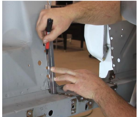
Figure 2 – Clearance Strut Tower Opening
