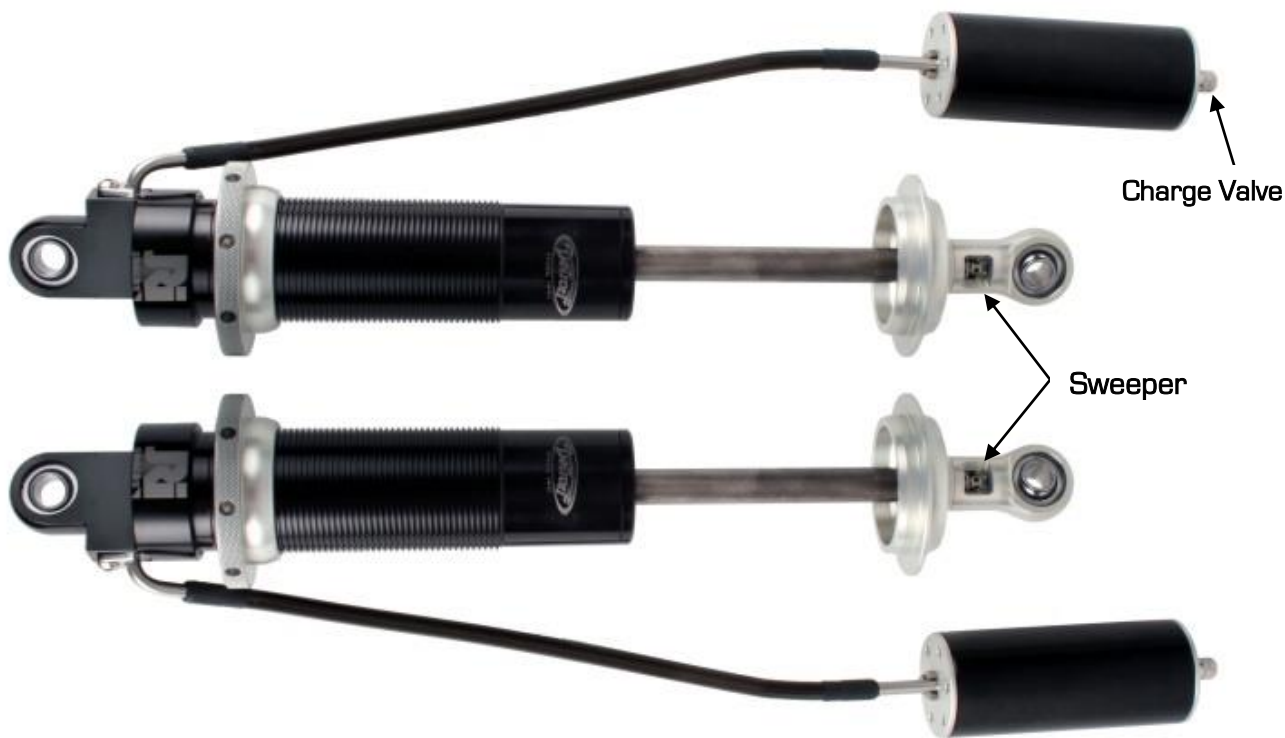
Figure 44a – Detroit Speed Double Adjustable Shock with Remote Canisters
