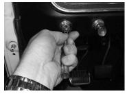
8) Place the dash spacer onto the end of the switch
