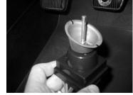
4) Push the wiper switch back and feed it out through the dash. Disconnect the connector from the switch body. Remove the dash spacer and set it aside.
