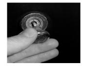
**7)** Now turn the ignition back on and test your new switch. You'll need to temporarily install the knob for this. If it works, proceed with the next steps. If not, check the connections.
