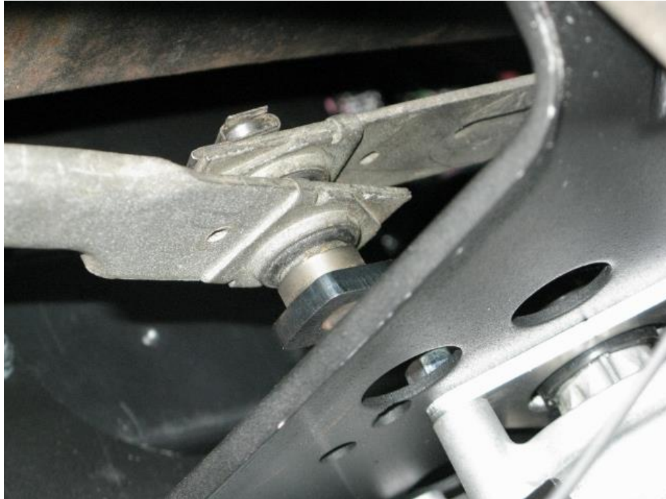
Figure 8 - Attach Wiper Linkage to Pitman Arm
