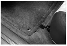
Reinstall the floor mat over the floor mat hook.
