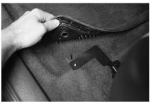
Option C: Use 1994-2004 Mustangstyle floor mat with a Ford floor mat hook. Purchase a Ford floor mat carpet hook (P/N 1W6Z76130A83AA), cut two slits into the carpet and install the floor mat hook. Choose one of the installation options for 1994-2004 Mustangs.
