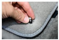
**Option A: Drill hole in existing floor mat and use supplied hardware.** Using the CarpetSaver bracket as a template, mark the floor mat for the hardware location. Drill a 17/64" hole in the floor mat and secure it using the supplied black stepped spacer and #10-32 button head cap screw.
