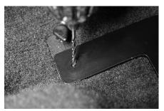
Making sure the end of the CarpetSaver bracket is squarely over the floor mat hook, use the bracket as a template and drill a 1/8" pilot hole into the carpet mat hook.
