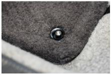
Option B: Use 1994-2004 Mustangstyle floor mat without a Ford floor mat hook. Install the supplied black stepped spacer and #10-32 button head cap screw directly into the CarpetSaver bracket. "Hook" a 1994-2004 floor mat over the hardware.
