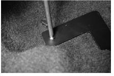
Use the #8 self-tapping screw to secure the CarpetSaver bracket to the floor mat hook.
